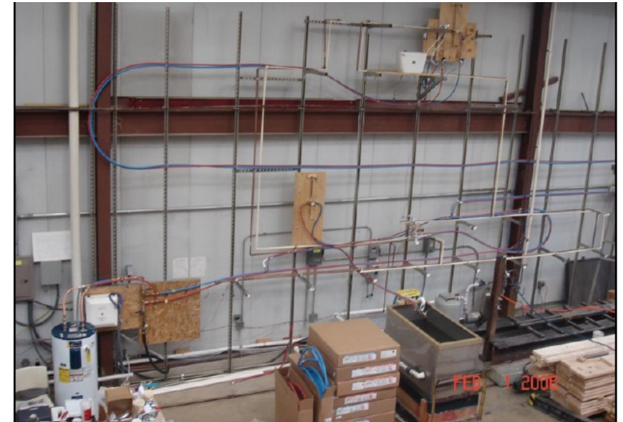
Figure 8.2 – Laboratory Test Set-up with Five Outlets, Hot Water Tank, and T&B System
